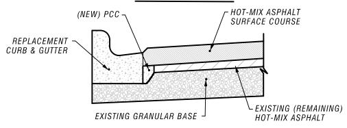
\* CURB & GUTTER SHALL BE SAWCUT (FULL DEPTH) PRIOR TO CURB & GUTTER SECTION.
